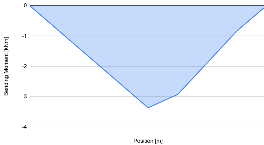
Figure 6.12 Shaft I Bending Moment diagram for Horizontal forces, used in analysis at center of shaft
